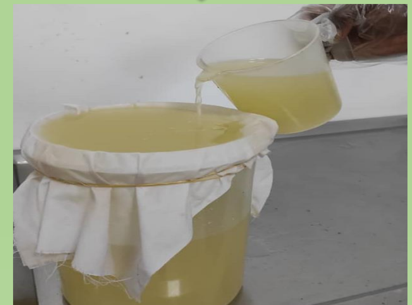
Filtration by a cotton cloth © Noel Dimoso
