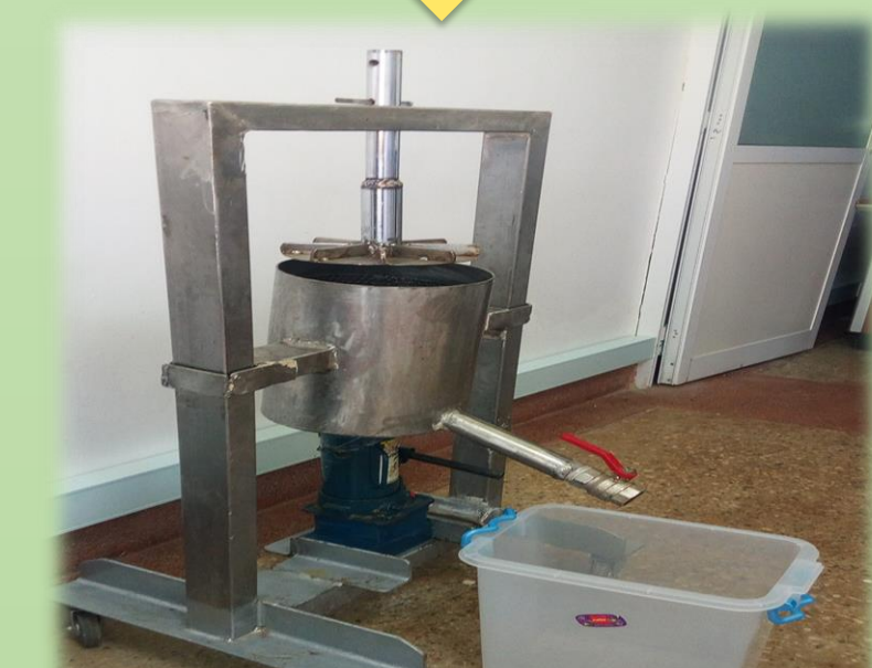
Hydraulic juice extractor © Noel Dimoso
